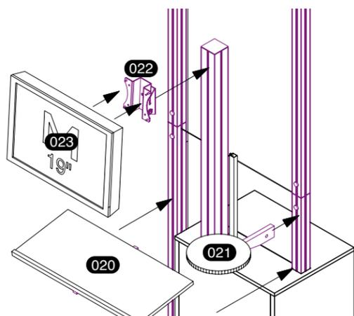
Connect monitor to center post as shown. Attach keyboard shelf and mouse shelf to smaller posts. Engage locks with supplied tool, tightening 1/4 turn to the right.
