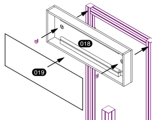
Connect lightbox (with lights pre-assembled inside) to the upper posts with supplied hammer-head bolts. Tighten with pliers or wrench (DO NOT OVERTIGHTEN).
